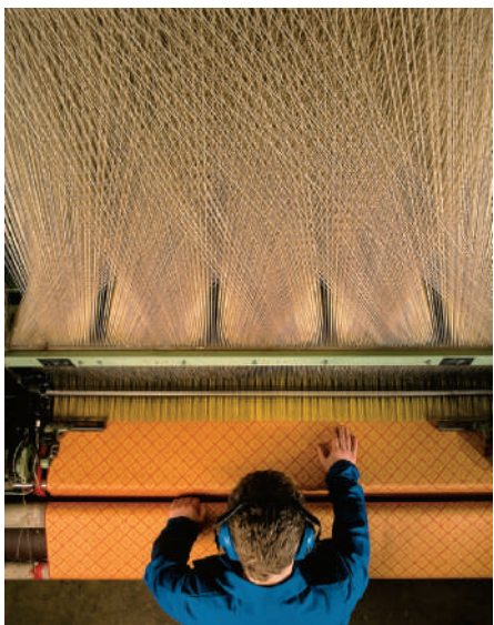
Figure 4-12. An industrial loom used to weave textiles.
